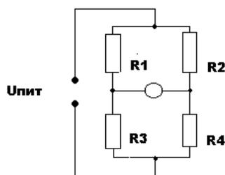
$$1. R_1 R_2 = R_3 R_4$$
